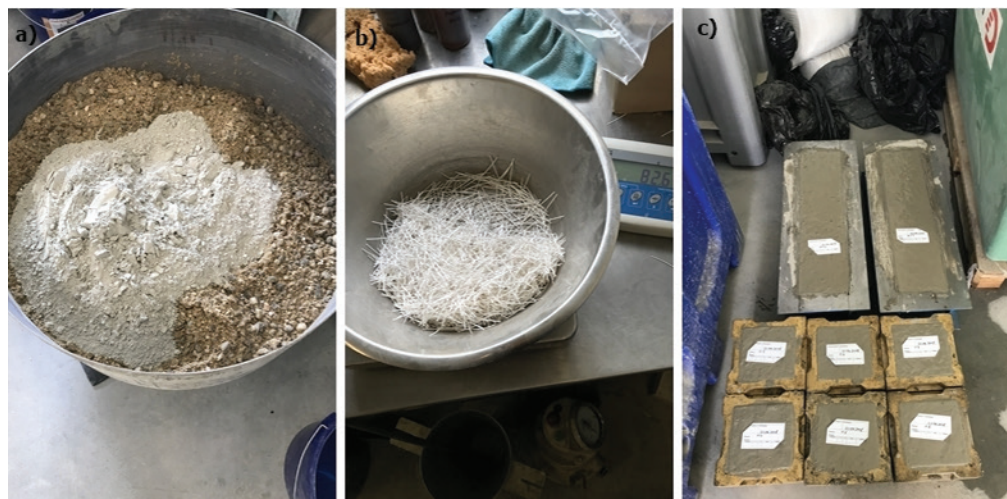
Fig. 2. Preparation of the concrete mixture: a) mixing of dry ingredients; b) weighing of the fibers; c) pouring concrete into the forms
