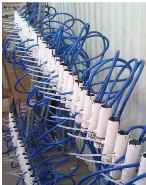
Fig 3. MCableS © multipoints temperature measurements cable (fot. Neostrain).
