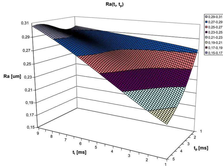
Fig. 5. Relationship between surface roughness parameter  $Ra$  and pulse and interval time  $Ra = f(t_i, t_p)$  when electrode feed rate  $v_f = 0.5$  mm/min, interelectrode voltage  $U = 19$  V, ultrasonic vibrations power  $P = 0$  W.
