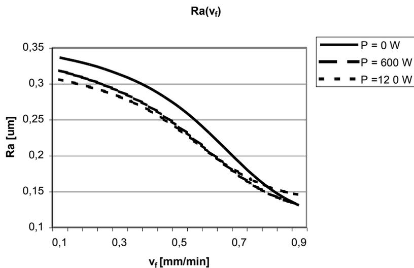
Fig. 10. Relationship between surface roughness parameter  $Ra$  and electrode-tool feed rate  $v_f$  for different power of ultrasonic vibrations when interelectrode voltage  $U = 19$  V, time of interval  $t_p = 3$  ms, time of pulse  $t_i = 5$  ms.
