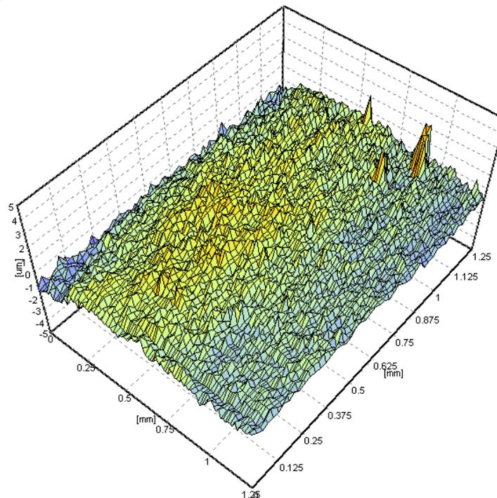
Fig. 12. Space surface geometrical structure after machining with electrode ultrasonic vibrations ( $P = 120$  W) when:  $v_f = 05$  mm/min,  $U = 19$  V,  $t_i = 5$  ms,  $t_p = 3$  ms; Space surface parameters:  $SP_p = 2.87$   $\mu\text{m}$ ,  $SP_v = 1.54$   $\mu\text{m}$ ,  $SP_z = 4.376$   $\mu\text{m}$ ,  $SP_a = 0.493$   $\mu\text{m}$ ,  $SP_q = 0.609$   $\mu\text{m}$ ,  $SP_{sk} = 1.567$ ,  $SP_{ku} = 2.922$
