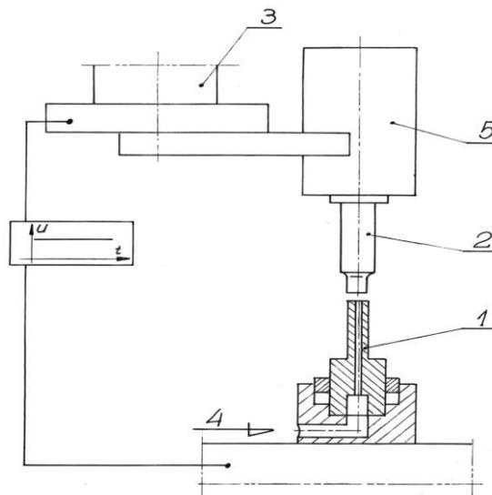
Fig.1. Scheme of test stand for investigations of PECM and USPECM process supported by electrode ultrasonic vibrations; 1 – workpiece, 2 – electrode - tool, 3 – tool plate of machine-tool EOCA 40, 4 – hole for electrolyte supplying, 5 – ultrasonic head.
