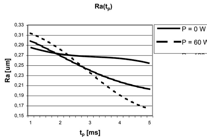
Fig. 8. Relationship between surface roughness parameter Ra and interval time  $t_p$  for different power of ultrasonic vibrations when pulse time  $t_i = 5$  ms, interelectrode voltage  $U = 19$  V, electrode - tool feed rate  $v_f = 0.5$  mm/min.
