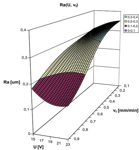
Fig. 6. Relationship between surface roughness parameter  $Ra$  and interelectrode voltage  $U$  and electrode-tool feed rate  $v_f$ :  $Ra = f(v_f, U)$  for pulse time  $t_i = 5$  ms and interval time  $t_p = 3$  ms when machining without electrode ultrasonic vibrations ( $P = 0$  W).
