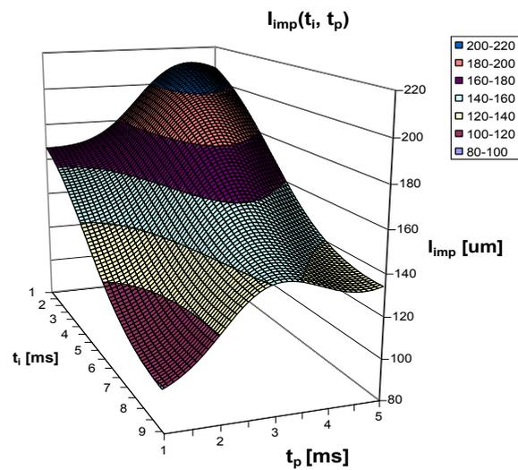
Fig. 4. Relationship between pulse and interval time  $I_{imp} = f(t_i, t_p)$  when electrode feed rate  $v_f = 0.5$  mm/min, interelectrode voltage  $U = 19$  V, ultrasonic vibrations power  $P = 0$  W.
