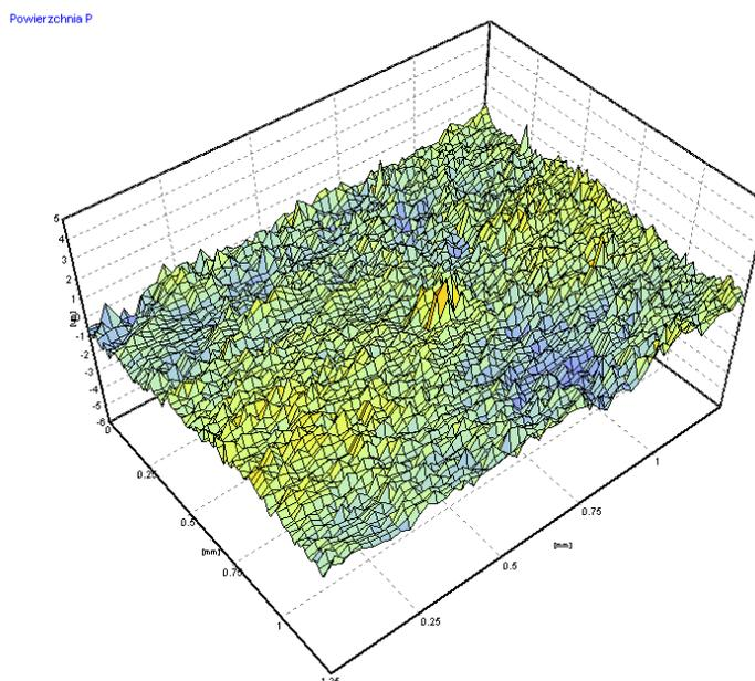
Fig. 11. Space surface geometrical structure after machining without electrode ultrasonic vibrations ( $P = 0$  W) when:  $v_f = 0.5$  mm/min,  $U = 19$  V,  $t_i = 5$  ms,  $t_p = 3$  ms; Space surface parameters:  $SPp = 2.577$   $\mu$ m,  $SPv = 1.56$   $\mu$ m,  $SPz = 4.137$   $\mu$ m,  $Spa = 0.337$   $\mu$ m,  $SPq = 0.428$   $\mu$ m,  $SPsk = 1.683$ ,  $SPku = 3.565$
