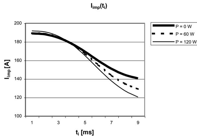
Fig. 7. Relationship between pulse current and pulse time for different power of ultrasonic vibrations when time of interval  $t_p = 3$  ms, interelectrode voltage  $U = 19$  V, electrode – tool feed rate  $v_f = 0.5$  mm/min.
