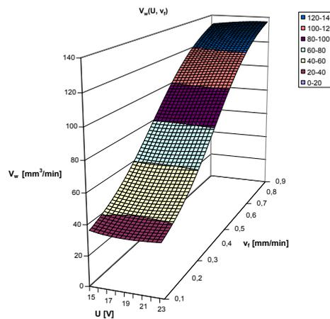
Fig.2. Relationship between metal removal rate and electrode tool-feed rate and interelectrode voltage  $V_w=f(v_f, U)$  for pulse time  $t_i = 5$  ms, time of interval  $t_p = 3$  ms when machining without electrode ultrasonic vibrations ( $P = 0$  W).
