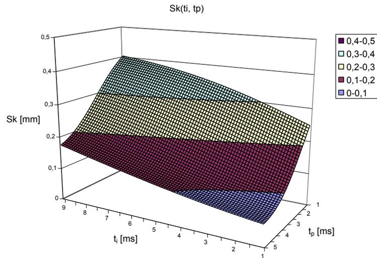
Fig. 3. Relationship between interelectrode gap thickness and pulse and interval time  $S_k = f(t_i, t_p)$  when electrode feed rate  $v_f = 0.5$  mm/min, interelectrode voltage  $U = 19$  V, ultrasonic vibrations power  $P = 0$  W.
