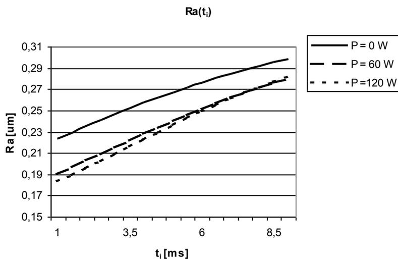
Fig. 9. Relationship between surface roughness parameter  $Ra$  and pulse time  $t_i$  for different power of ultrasonic vibrations when interelectrode voltage  $U = 19$  V, time of interval  $t_p = 3$  ms, electrode – tool feed rate  $v_f = 0.5$  mm/min.
