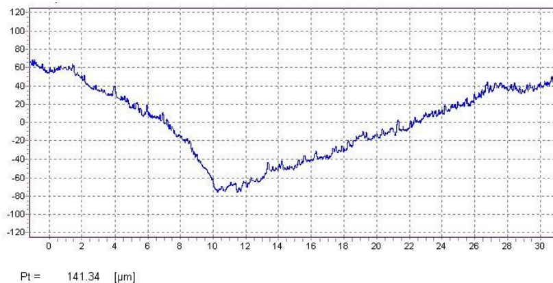
Fig. 8. Surface geometrical structure after electrochemical smoothing; D = 0,280 mm, V_f = 0.1 mm/min, g \sim D , P_t = 141.34 \mu\text{m} .
