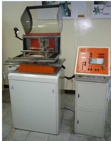
Fig. 1. Picture of the workstation consisting of electroerosion wire cutter BP – 95d and transistor pulse generator
