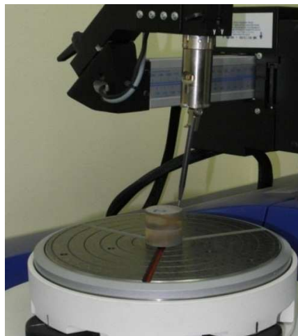
Fig. 9. Close-up the rotational table along with cylinders during measurement
