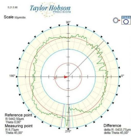
Fig. 13. Polar graphs and outline of roundness deviations of the cylinder at height: 7 [mm]
