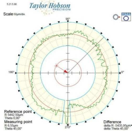
Fig. 12. Polar graphs and outline of roundness deviations of the cylinder at height: 1 [mm]
