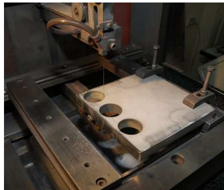
Fig. 2. Way of mounting processed material, from which cylinders were cut
