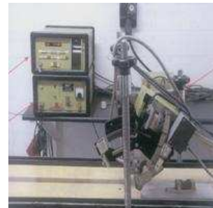
Fig. 6. Strainflex PSF 2M device for stress measurement: a general view
