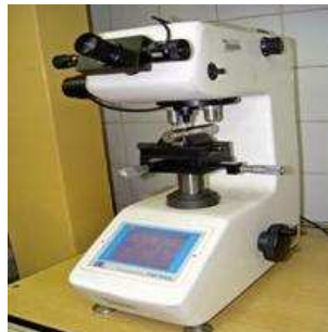
Fig. 5. FutureTech FM700e microhardness tester: a general view
