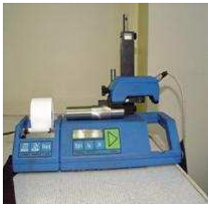
Fig. 4. Hommeltester T1000E profile measurement gauge: a general view
