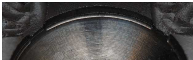
Fig. 8. The tool path after pencil machining of residual material
