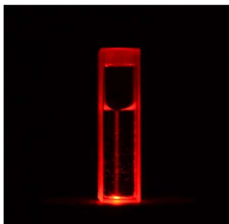
Figure 8. Passing laser pointer beam through the guanine solution.
