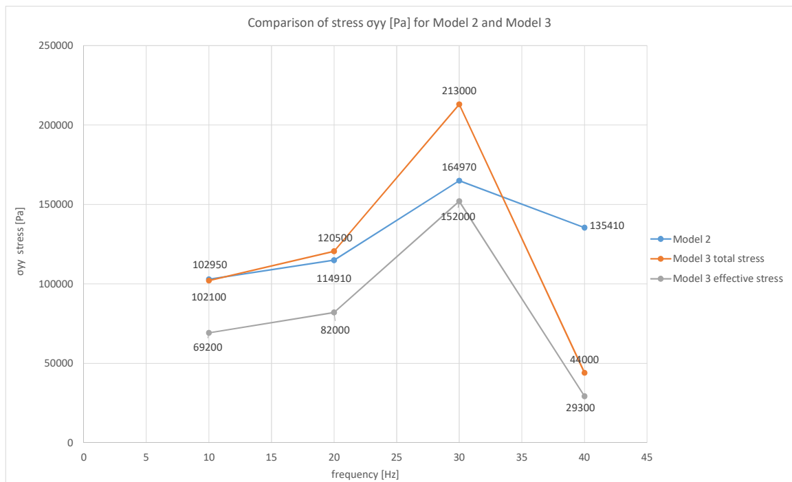
Fig. 6.32: The comparison of Soil Type 1 stresses in the vertical direction for the sample point for four arbitrarily chosen frequencies -10,20,30 and 40Hz, for two analyzed models.
