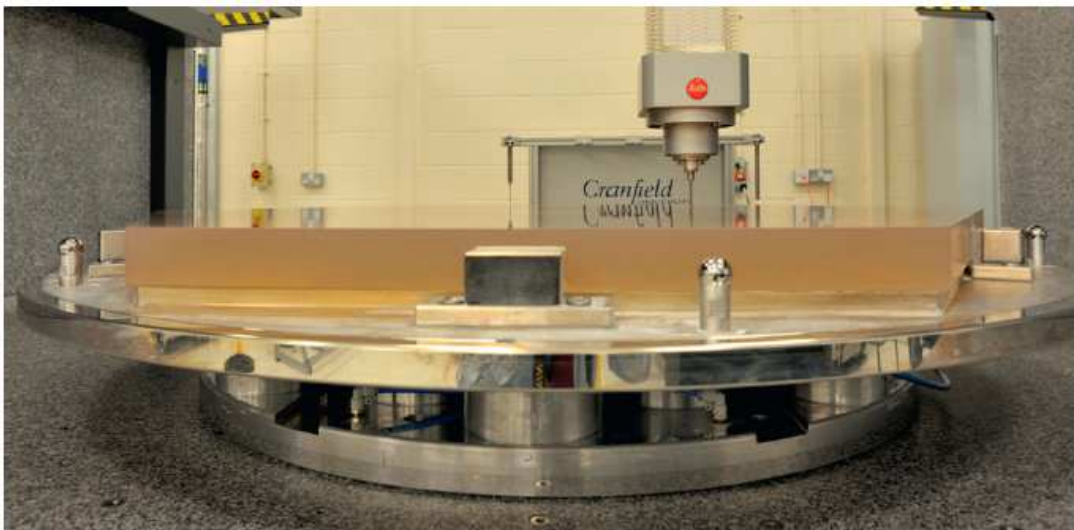
Figure 8 Post-Process Audit Measurement using a LEITZ PMM-F 30.20.10 / LSP-S4 (Low Force Probing) ; MPE_E 1,7+L/400m
