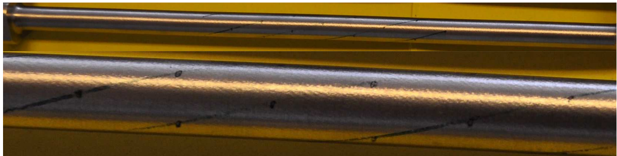
Figure 5.17. Deformation of sample 3 after 870°, together with a magnified view of the lines which were initially parallel
