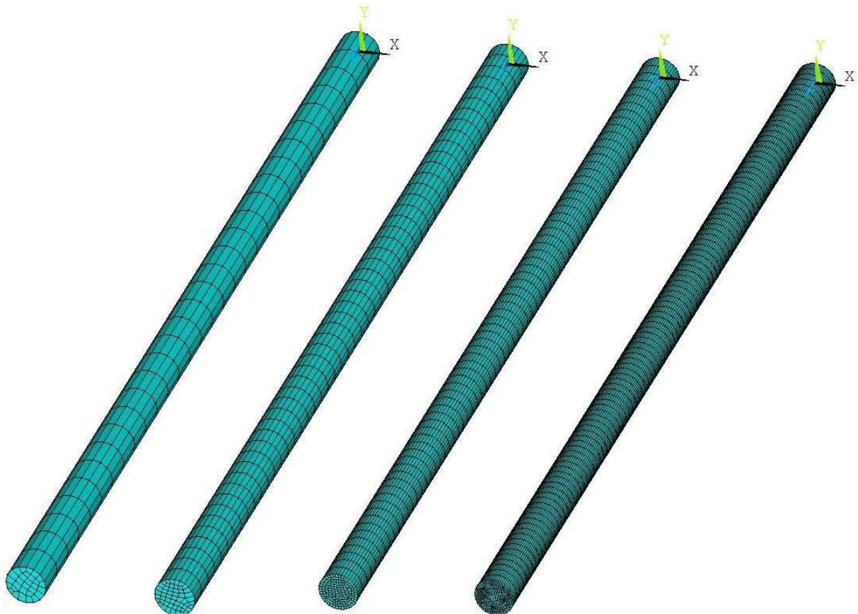
Figure 13.6. Column mesh, from left to right: mesh 1 & 5, mesh 2 & 6, mesh 3 & 7, mesh 4
