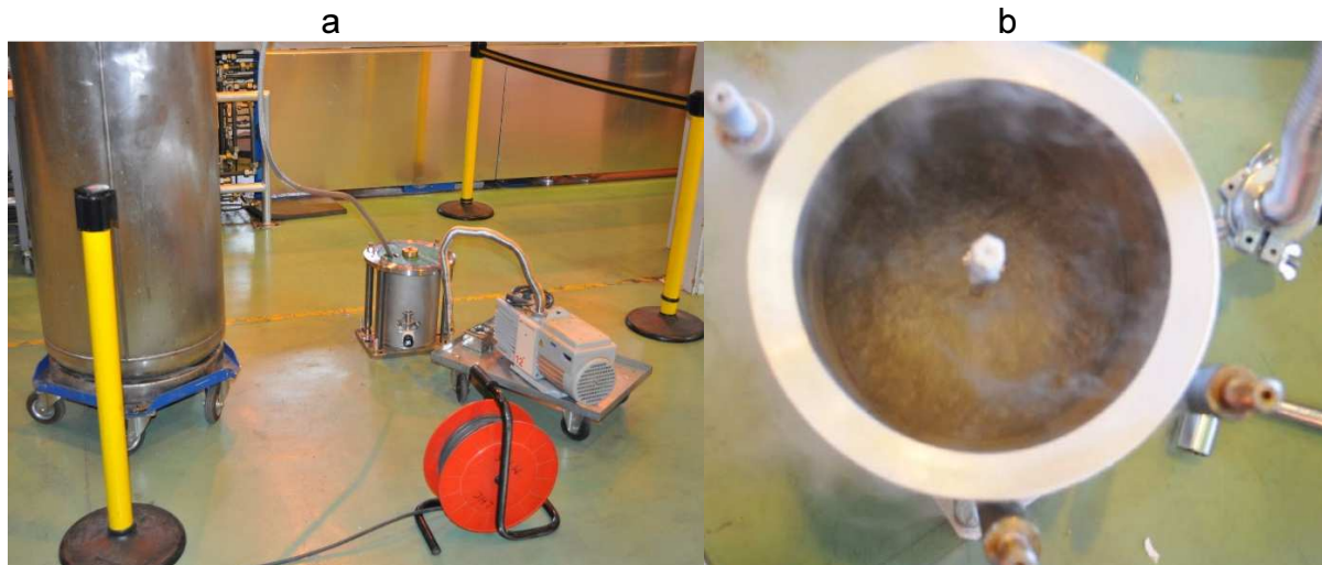
Figure 7.1. a) Set-up with the vacuum pump and the liquid nitrogen dewar , b) sample immersed in the boiling nitrogen
