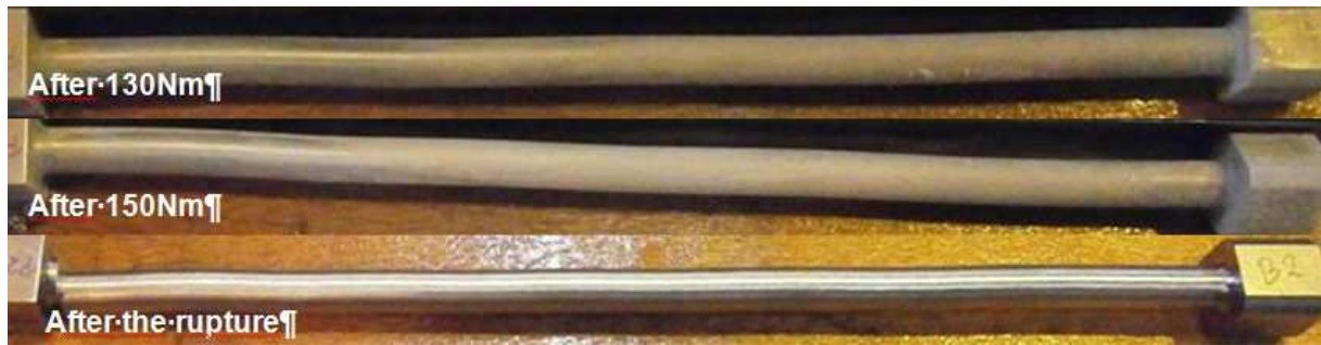
Figure 7.35. Deformation of sample 7.2 twisted at 77K
