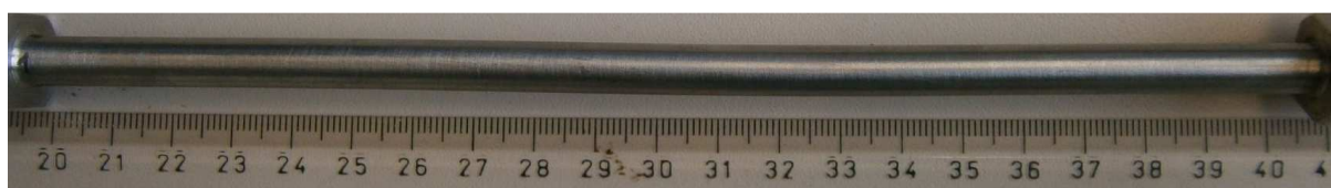
Figure 11.12. Sample A10 after cyclic torsion at 77K, before tensile test
