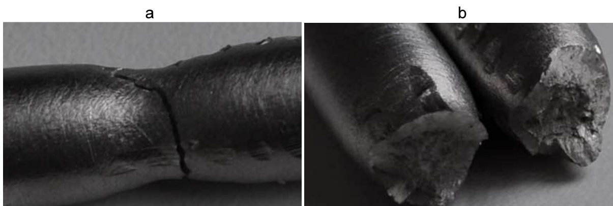
Figure 11.46. Magnified fracture zone for sample 62, a) side view, b) front view
