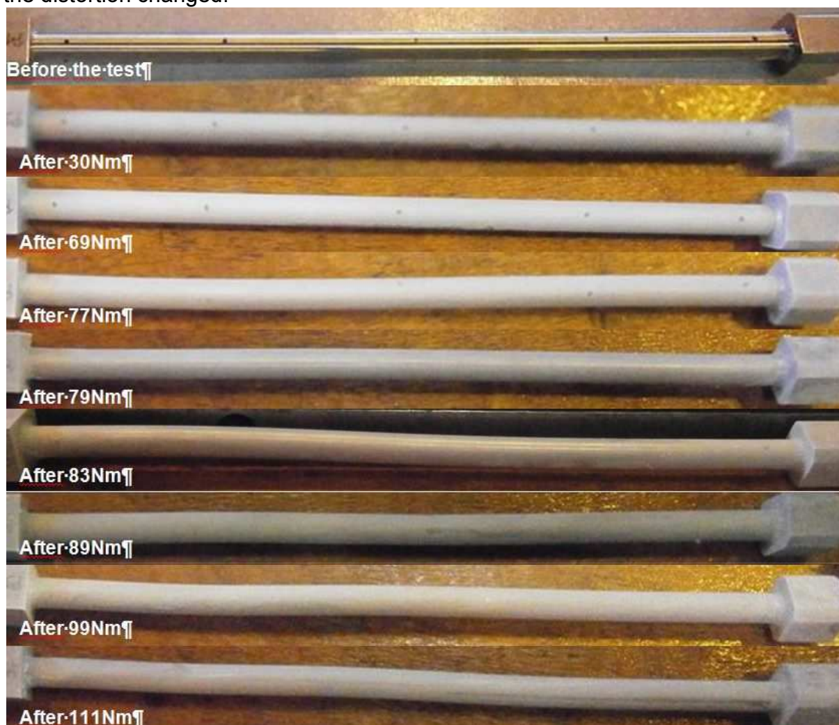
Figure 7.31. Deformation of sample 7.1 twisted at 77K
