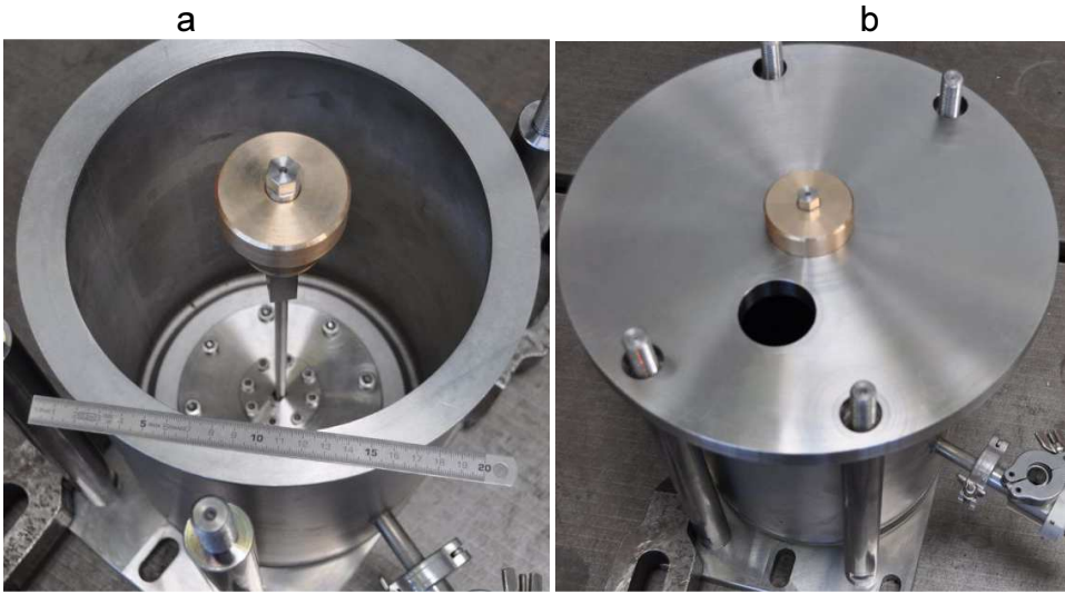
Figure 5.2. a) The interior of the cryostat with sample and bushing; b) The set-up with top flange
