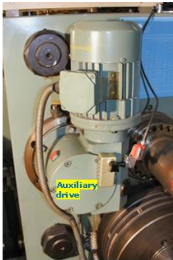
Figure 22 Tool Movement / Four Eccentric Shafts/Left Auxiliary Drive
