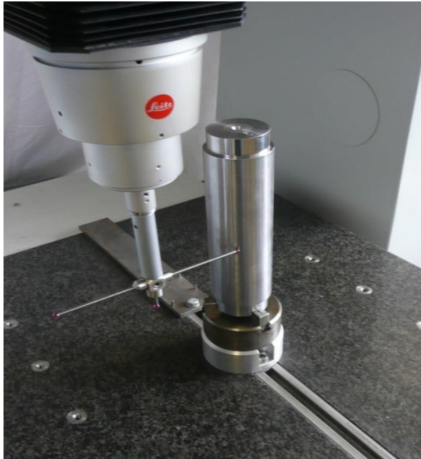
Figure 49 Clamping situation blank / measuring machine table
