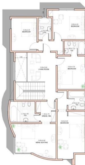
AREA = 186 SQ. M. FIRST FLOOR PLAN SCALE 1:100
