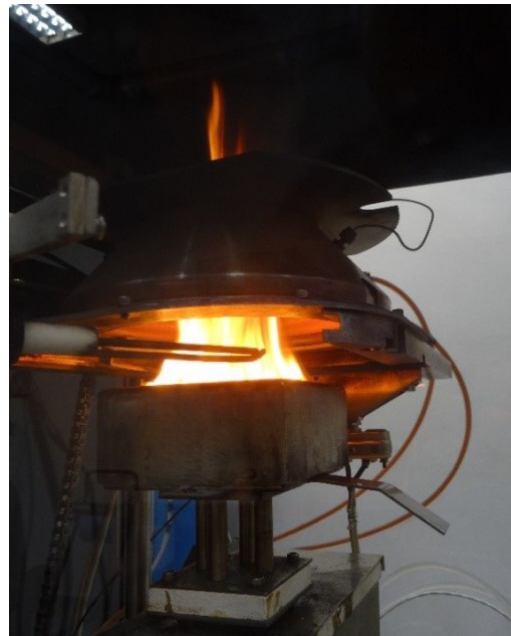
Fig. 3. The sample during test in Railway Institute according to ISO 5660-2
