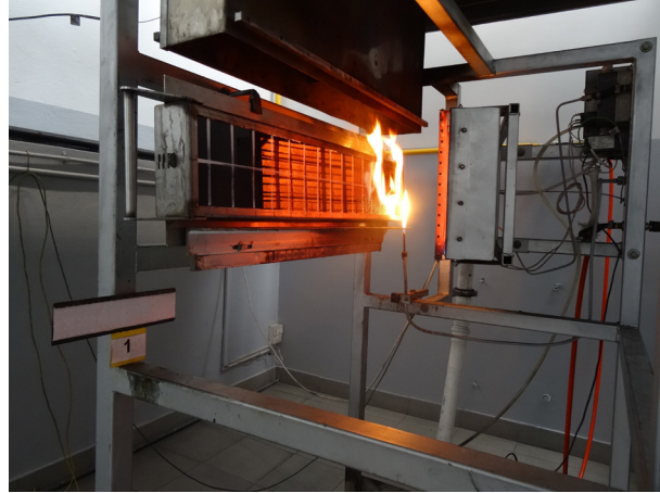
Fig. 2. The sample during test in Railway Institute according to ISO 5658-2
