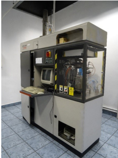
Fig. 3. The sample during test in Railway Institute according to ISO 5660-2
