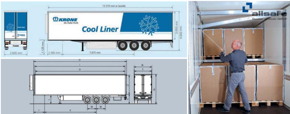
Fig. 3. Dimensions of Krone Cool Liner cooling semi-trailer with ATD II system
