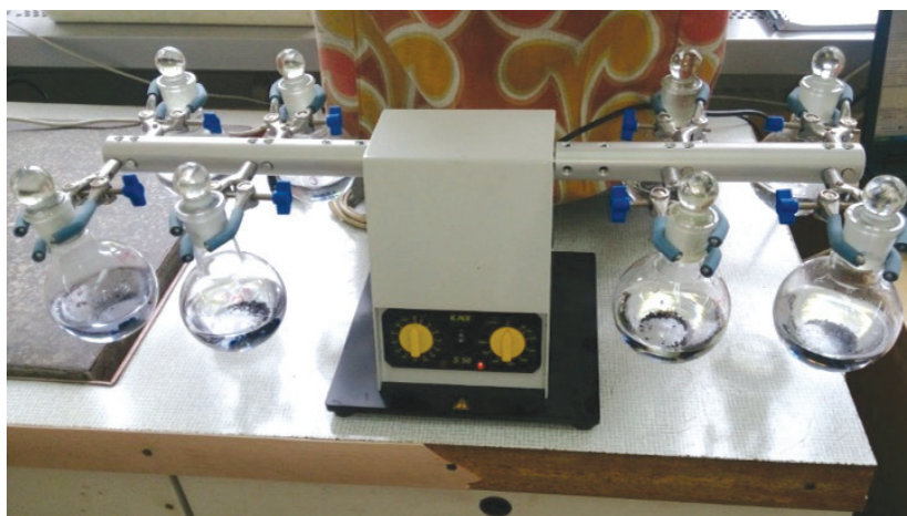
Fig. 2. Flat bottom flasks placed in a shaker during equilibrium measurements
