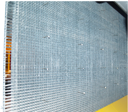
Fig. 5. Distribution of the measurement points at the inlet to the wind tunnel scheme (a), view in the wind tunnel (b)
