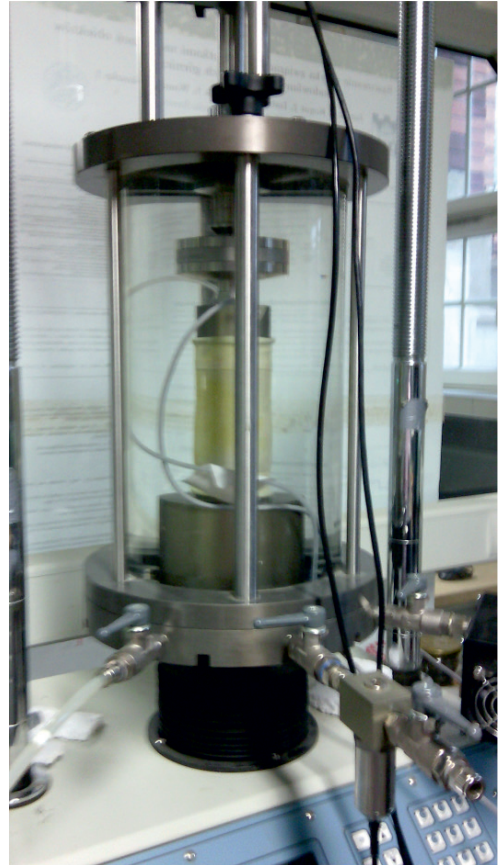
Fig. 3. Bender elements, mounted on the base of the apparatus (a) and located directly in the polycarbonate chamber during triaxial stress testing (b), used for the testing of wave propagation under laboratory conditions
