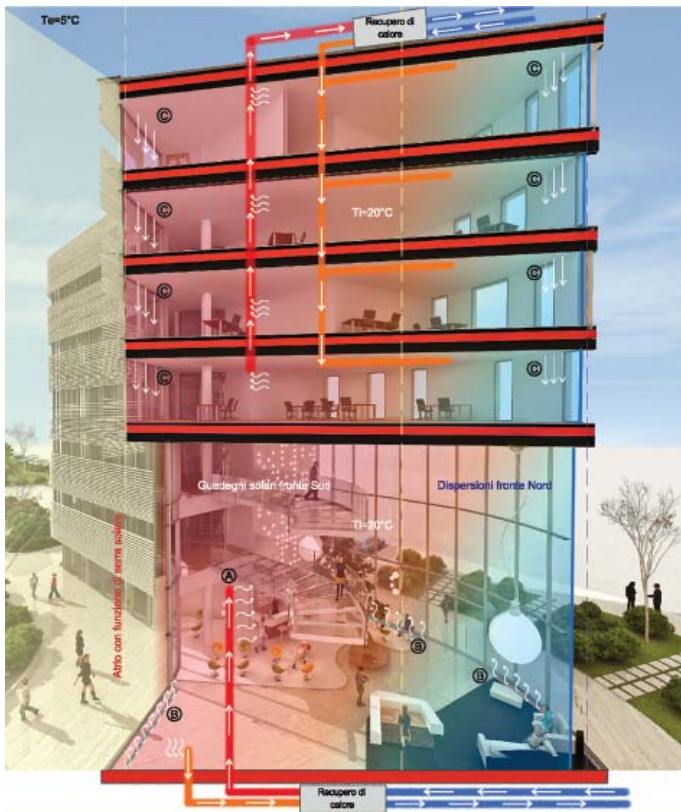
ill. 19: representation on top of Revit 3D section, of the management of thermal equilibrium of the building during winter. (Credits: courtesy ATlproject)
