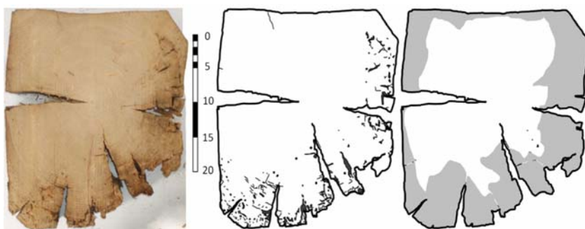
Fig. 7. Post-autopsy view of health situation of beam cross-section (legend in centimetres, left), distribution of insects attack on section surface (centre), decay distribution due to brown rot (right)
