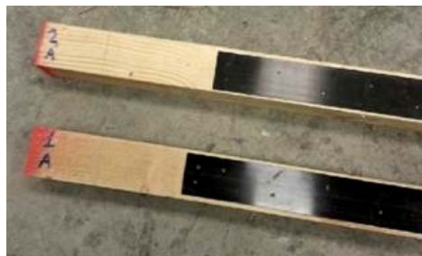
Fig. 3. Detail of application of the CFRP plate
