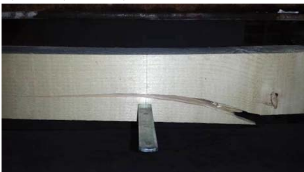
Fig. 11. Typical tensile failure mode of unreinforced beams near a knot or due to grain deviation
