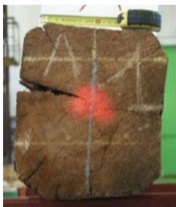
Fig. 1. Beam end view (left), geometric survey of tested cross-section (centre); tomographic stations along the perimeter (right)
