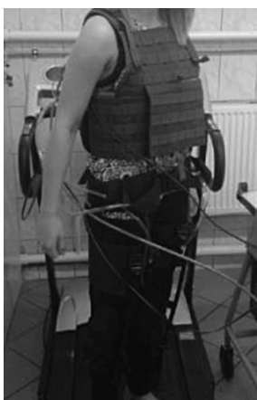
Fig. 2. A flexible suit supporting a motion motoric driven by McKibben PAMs
