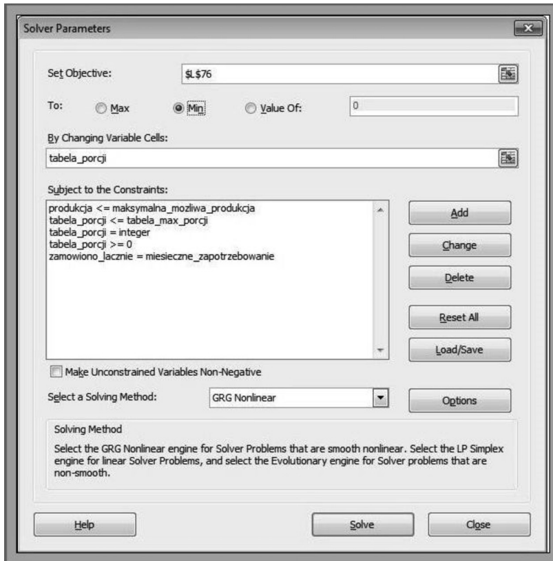
Fig. 18. The Excel Solver add-in dialogue box – the concrete plant’s chain ordering policy
