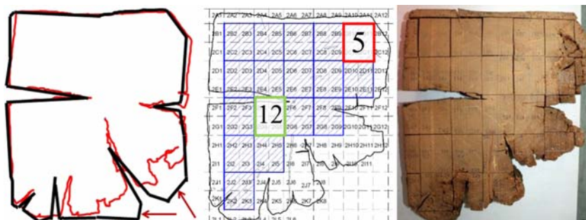
Fig. 8. Comparison between section perimeter from survey at time of tomography data collection (in black) and geometry after cutting of timber (in red); arrows point to material loss between the two phases (left). Grid of specimens for compression tests with position of specimens 5 and 12 (centre). Slice after specimens' cutting (right)
