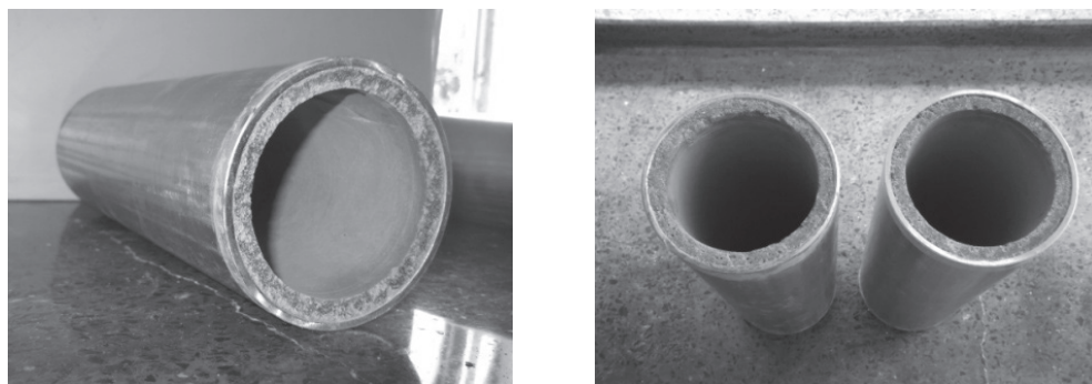
Fig. 2. Steel pipes with internal cement coating (Source: author's photo)
