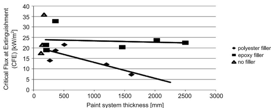
Fig. 3. Test results of *Critical Flux at Extinguishment (CFE)* [kW/m<sup>2</sup>] of surface protection systems for rolling stock (archive IK, 2014–2015)
