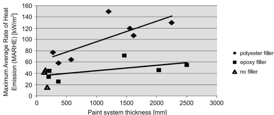
Fig. 2. Test results of *Maximum Average Rate of Heat Emission (MARHE)* [kW/m<sup>2</sup>] of surface protection systems for rolling stock (archive IK, 2014–2015)
