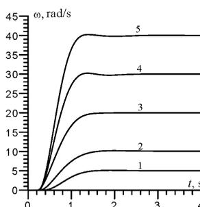
Fig. 6. The transient process' curves of motor's angular speed for constant meaning  $\omega_{\text{fixed}} = 5$  rad/s, (curve 1), 10 rad/s (curve 2), 20 rad/s (curve 3), 30 rad/s, (curve 4), 40 rad/s, (curve 5)
