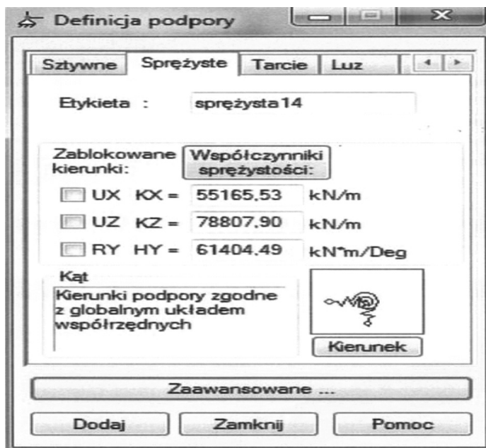
Fig. 2. The definition of the elastic support in Robot
