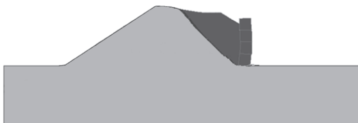
Fig. 4. Sliding surface for embankment with 4 gabions
