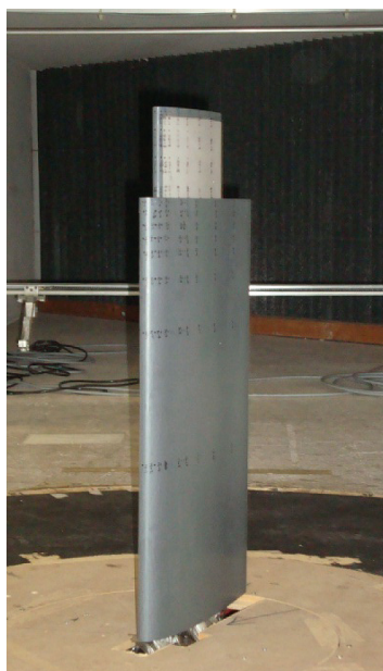
Fig. 14. Photograph of larger pressure tapped model stepped blade in the wind tunnel
