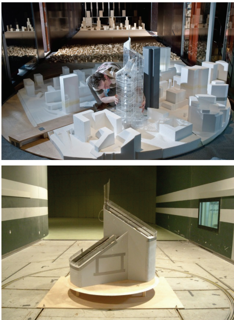
Fig. 3. High rise building scaled 1/200 in BLWT (top) and model of the top of the same tower at a 1/50 scale in a high-speed wind tunnel (bottom) for measurements at a high Reynolds number
