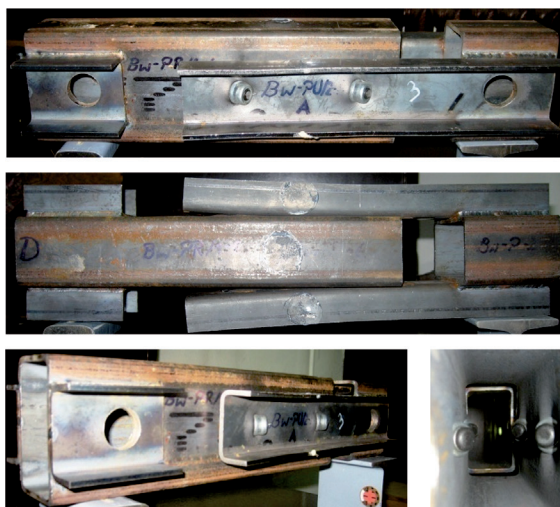
Fig. 13. Typical failure mode of the specimen after unloading
