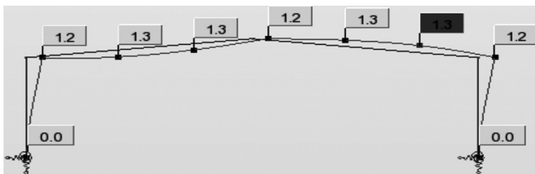
Fig. 3. First mode shape of variant I
