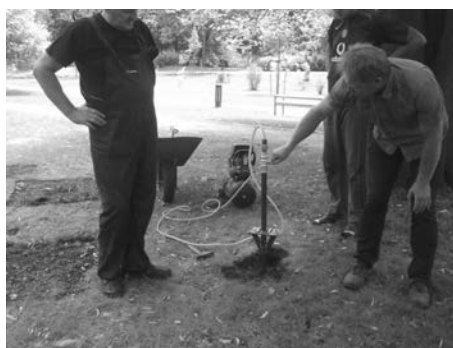
Ill. 7. Device for soil aeration
