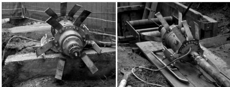
Fig. 2. Rotary head for cement mortar lining water pipes (author's photo)
