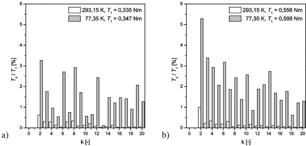
Fig. 8. Higher harmonics of electromagnetic torque  $T_k$  in relation to the first harmonic  $T_1$  for: a)  $i_a = 3$  A, b)  $i_a = 5$  A measured at room temperature and at liquid nitrogen temperature
