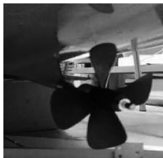
Fig. 6. Propeller, diameter 9 cm
