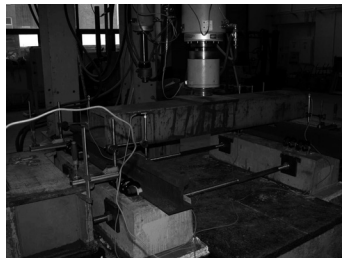
Fig. 2. LONGASF sample with ICOSTRUN 03 during stiffness tests [1]
