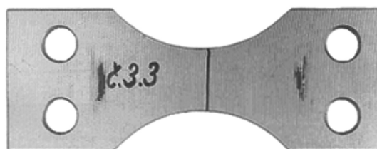
Fig. 5. The shape of a test body for the bending fatigue strength test of different machining technologies
