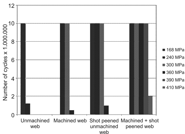
Fig. 9. Comparison of stress levels of railway wheels with different final finishing of the wheel web
