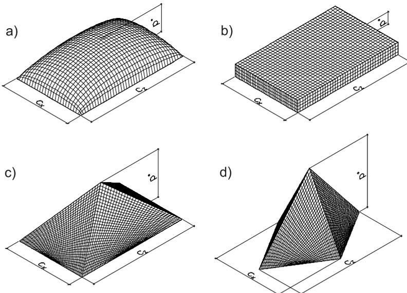
Fig. 3. Pressure distributions used in parametric study
