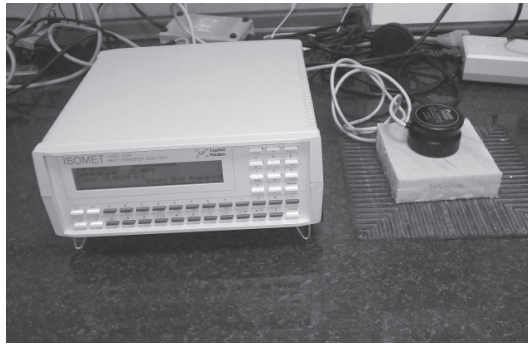
III. 2. Measurement of thermal parameters
