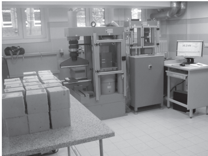
III. 3. Measurement of compressive strength
