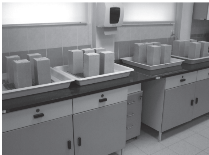
III. 1. Measurements of water sorption coefficients
