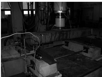
Fig. 2. LONGASF sample with ICOSTRUN 03 during stiffness tests [1]
