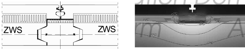
Fig. 4. Panel joint. Temperature distribution in the panel connection (from AnTherm program)
