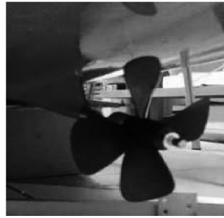
Fig. 6. Propeller, diameter 9 cm
