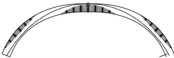
Fig. 7 The arch at 2 mm horizontal yield of the right abutment (scale factor 200). Plastic hinge at apex
