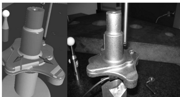
Fig. 3. Measurement programmed using I++ Simulator (left side) transferred and performed on PMM 12106 machine (right side)
