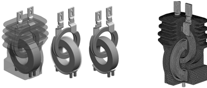
Fig. 4. Geometry of current transformer (left) and its discretization in ABAQUS (right)
