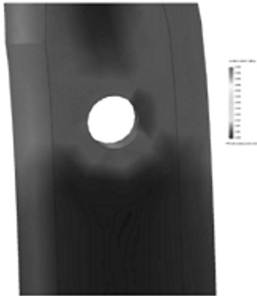
Fig. 3. Detailed image of stress distribution in fixing bond
