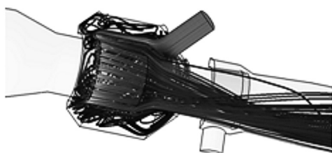
Fig. 2. Path lines of motive liquid
