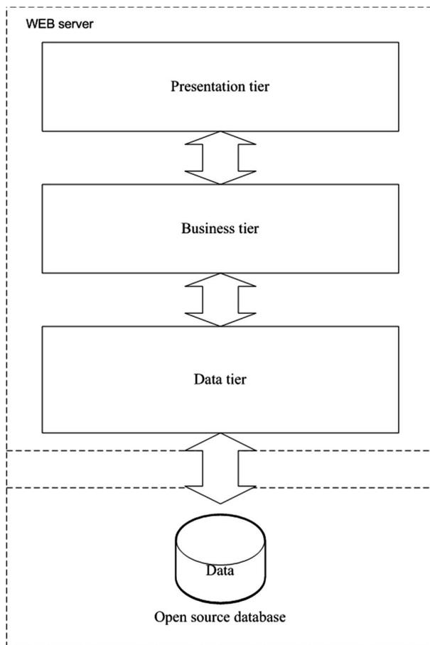
Fig. 3. Open source database server in three-tier architecture
