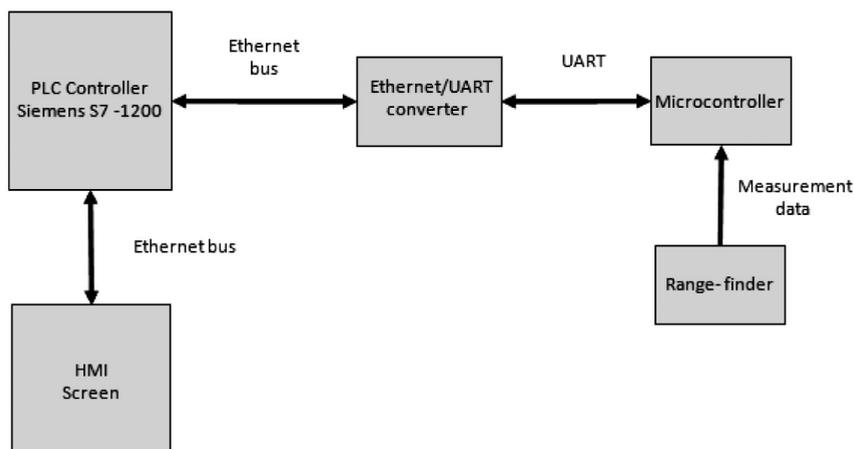
Fig. 1. The block diagram of the proposed system
