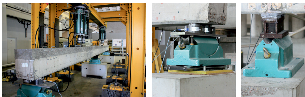
Fig. 6. Photos of the test stand, extreme and intermediate supports
