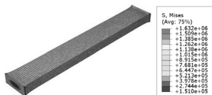
Fig. 5. Cauchy stress distribution corresponding to the nominal strain of 30% in polymer verification of the FEM model of the dumbbell specimen
