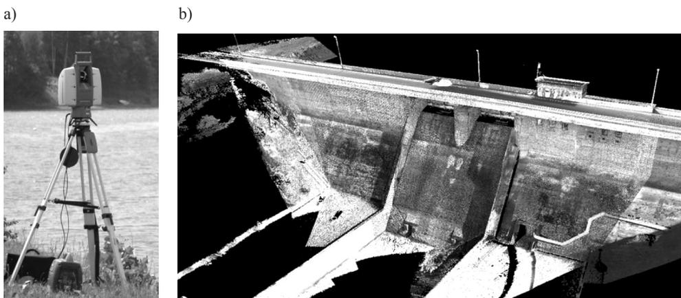
Fig. 1. Measurements of the Besko Dam. a) Leica Scanstation 2 scanner during surveys, b) results of surveys of the dam from the downstream face – results of combination of 5 clouds (about 155 million points)
