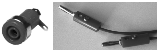
Fig. 3. The panel mounting a banana socket (left) and the wire with banana plugs (right)
