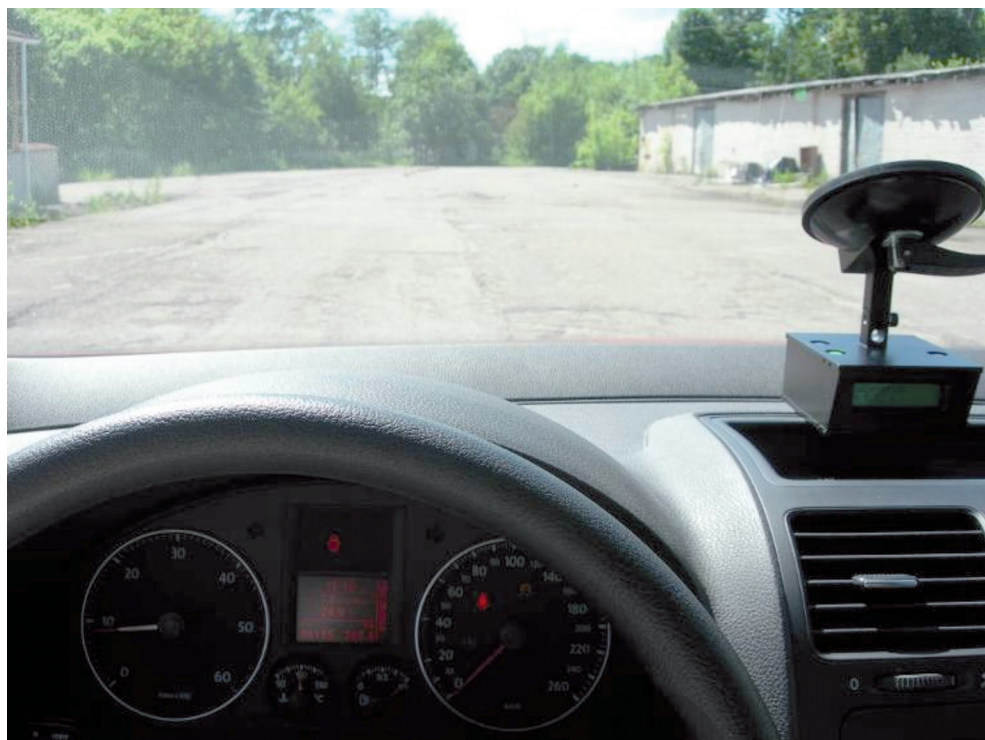
Fig. 1. The experimental road sector with a dry asphalt-concrete pavement (the accelerometer installed in the car)
