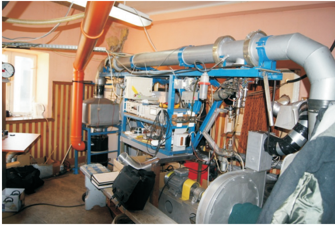
Photo 3. General view of the measurement stand for determining the emission of particulate matters with a tunnel diluting the exhaust gases
