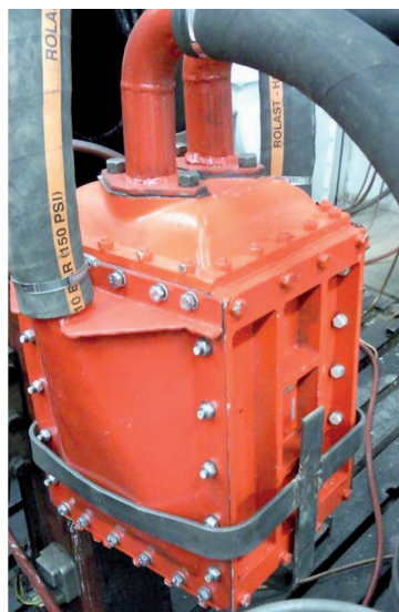
Fig. 1. Intercoolers: air/air type – left side, water/air type – right side
