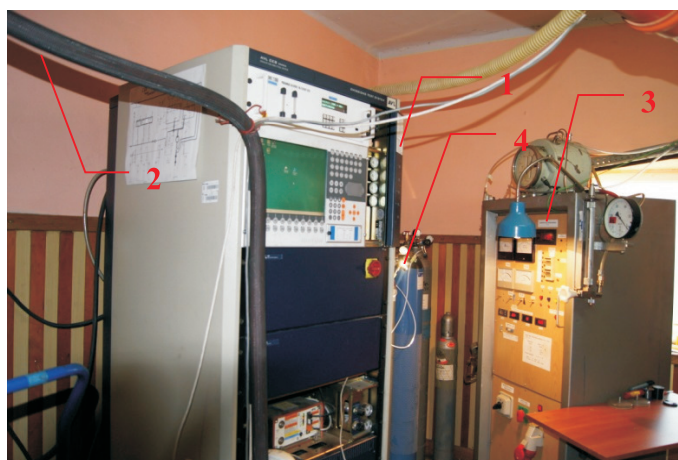
Photo 2. Test stand for determining the emission of exhaust components – type CEB II of the firm AVL, used in the investigation: 1 – Set of analysers CEB II of AVL (Austria), 2 – Heated line for exhaust sampling, 3 – Set of 8 cylinders with calibrating and working gases, 4 – Stand controlling the settings of the tunnel diluting exhaust gases (measurement of particulate matters)
